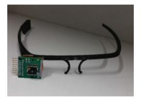
**Figure 3:** Miniature FLIR lepton thermal camera attached to a 3D printed glass, envisioning the potential form factor.
